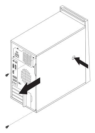
Figure 5. Removing the computer cover
